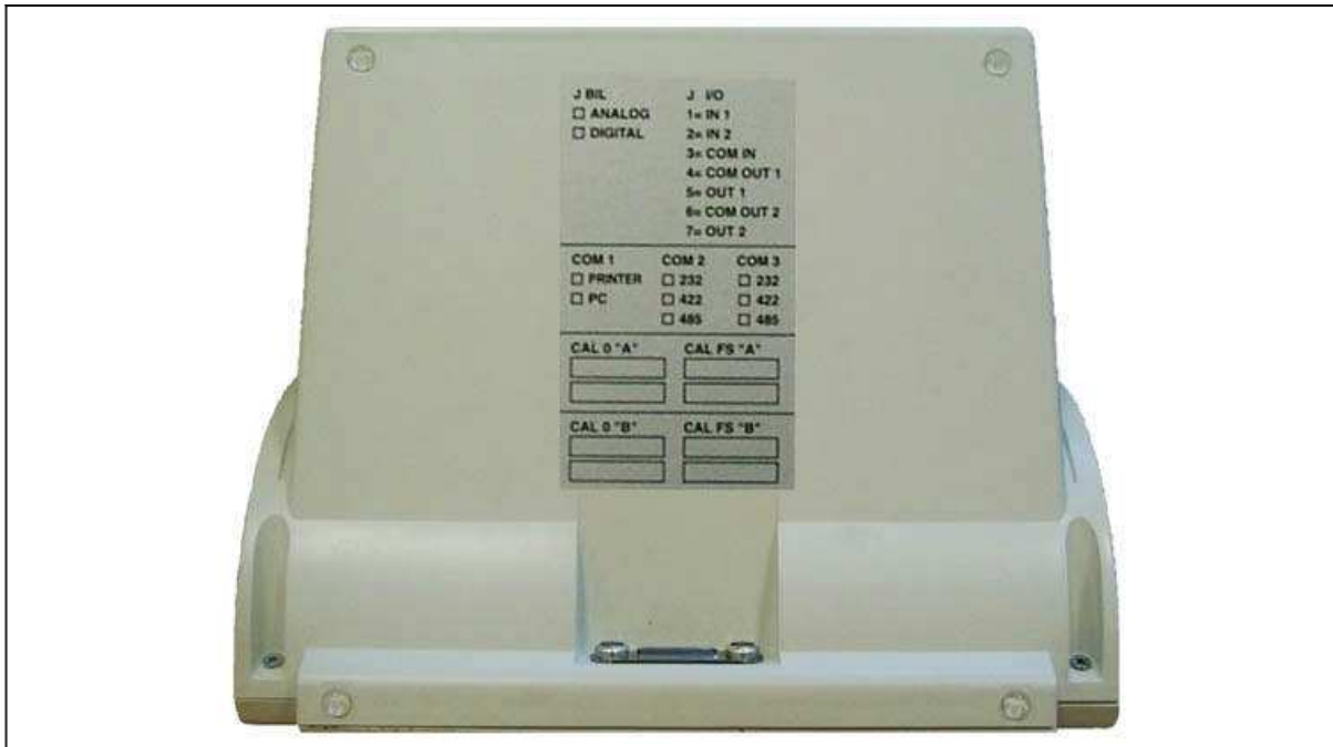
Figure 8.1 - Outputs identification label on base of terminal (citi0410.jpg)
